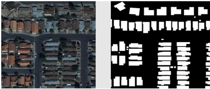
Fig. 2. An example of images (left) and labels (right) in the SpaceNet Building Detection V2. [1]
